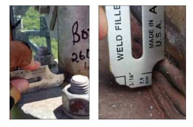
**Weld profiles** should meet the visual acceptance criteria as specified in Tables 8.1. Welds should be free from cracks, overlaps, and unacceptable profile discontinuities
