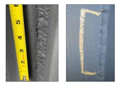
**Underfill** is a groove weld condition in which the weld face or root surface is below the adjacent surface of the base metal. In essence, the joint has not been completely filled with weld metal and is incomplete.
