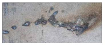
**Crater** is a depression in the weld face at the termination of a weld bead. The Code's Table 8.1 requires all craters to be filled to provide the specified weld size, except for the ends of intermittent fillet welds outside of their effective length.
