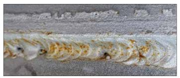
**Inclusion** is defined as entrapped foreign solid material, such as slag, flux, tungsten, or oxide. When it comes to tower and monopole upgrades, typically inclusion is slag left within a complete joint penetration (CJP) weld and is located by a post-modification ultrasonic testing (UT) non-destructive examination. Slag inclusions result from improper welding technique, lack of access, or improper cleaning between weld passes.
