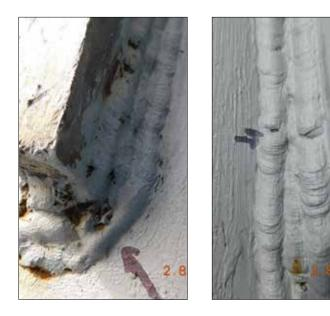
**Incomplete joint penetration** is a joint root condition in which the weld metal does not extend through the joint thickness. In other words, the weld does not penetrate into the root area of the weld. Typically, this condition is identified via UT non-destructive weld examination.
