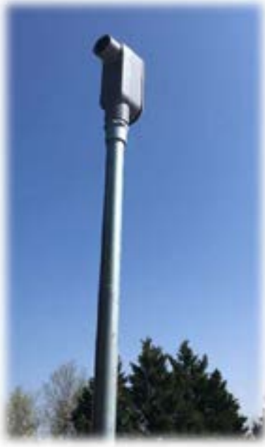
Photodiode sealed from water intrusion facing northern sky (in Northern Hemisphere)
