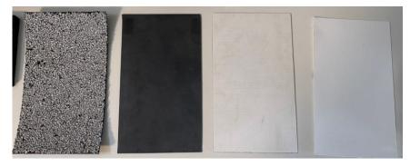
• Two (2) different types of typical rubber mats that are recommended to be used under rooftop ballast mounts:
